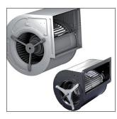
Radial impellers of high performance balanced statically and dynamically, type 2, 5 according to DIN/ISO 1940. Extremely silent and vibrations free. The speed control is obtained through an electronic selector and a 5 stage converter, integrated within the box.
