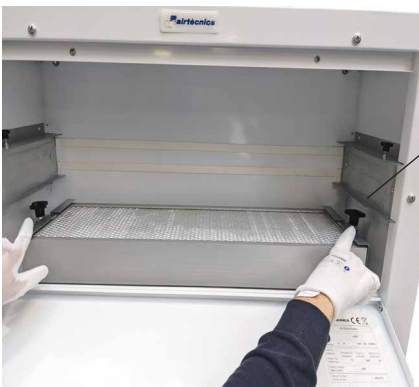
5- Loosen the threaded knobs and staples of the absolute
