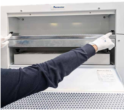
3- Loosen the threaded knobs on the pre-filter.
