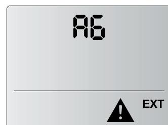
Stops and locks the unit. To unlock it, the power supply must be switched off. It is activated with DIN3 digital IN on the control unit.
